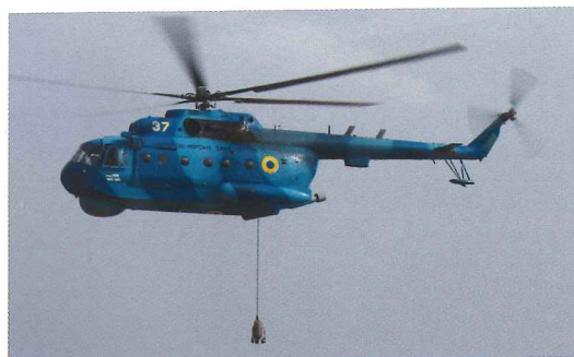
One of the Mi-14 helicopters shows its dipping sonar, used to detect and track submarines
