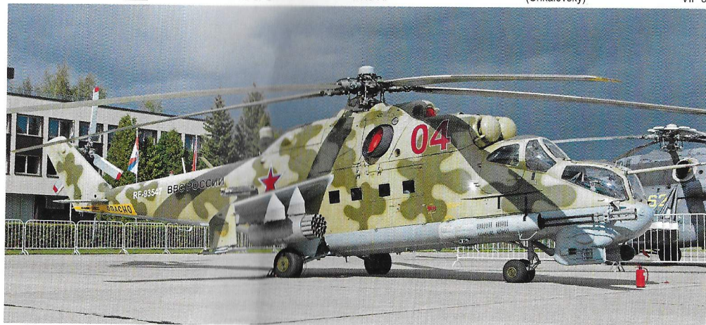
In addition to several new Mi-35Ms a nice appearance at Army 2016 was this veteran Mi-24P which can be identified by its fixed gun mounted on the right side of the fuselage. (Kubinka, 8 September 2016, Paul van der Linden)
