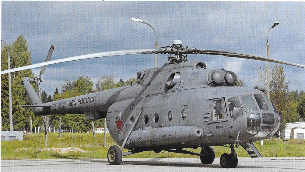
The Mi-8 is a challenging type for recognition of the exact subtype. Various types could be seen during Army, including this older Mi-8MTV RF-19030. However, the difference between MTV-subtypes is hardly visible. The construction number can help with this, but it is usually hard to find. With this one, the c/n is on the engine intake-cones. (Kubinka, 8 September 2016, Paul van der Linden)
