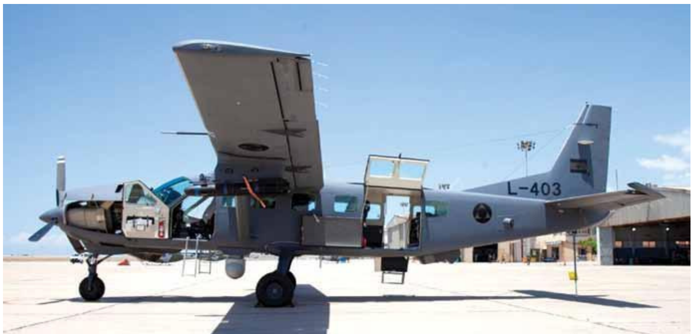
4 Squadron at Beirut was majorly involved in the Qalamoun offensive, their three AC-208 Combat Caravans proving a valuable asset. The AC-208 can carry two Hellfire missiles and is equipped with high-tech equipment for its ISR missions. Photo: Stefan Goossens
