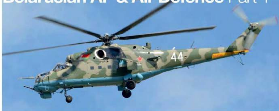
Above: The remaining Mi-24s were all assigned to the 50th Mixed Aviation Base after the airfield at Pruzhany was closed during the air force's latest reforms. This example, '44 White', is a Mi-24K 'Hind-G2' intended for artillery spotting and combat reconnaissance, with no guided-missile systems. Erwin van Dijkman Below: The MiG-23 was one of the first types withdrawn from use after independence. In 2001, 31 MiG-23MLDs and six MiG-23UBs were still in service at Baranovichi and were retired soon after. Most were scrapped or sold abroad, but '88 White' is stored at Minsk-Lipki.
