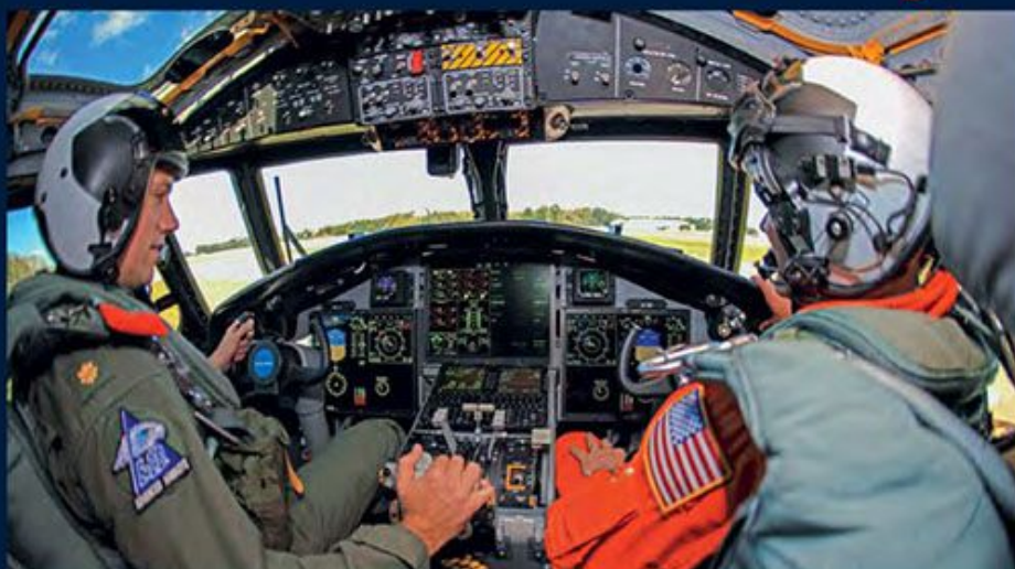
Above: Inside the glass cockpit of an E-2D at Saint Augustine, Florida. On the left is LCDR Drew 'Balls' Ballinger and on the right is Tom 'Booty' Boutin. The E-2D co-pilot can also perform radar mission tasks, rather than just help fly the aircraft. Below: LT Dave 'Cabbage' Peterson working in the back of an E-2D. The Advanced Hawkeye has the more capable and further-reaching AN/APY-9 radar. The fully digital phased-array radar has demonstrated the ability to detect small targets, such as cruise missiles, at greater ranges than its predecessor, and also offers improved stability.
