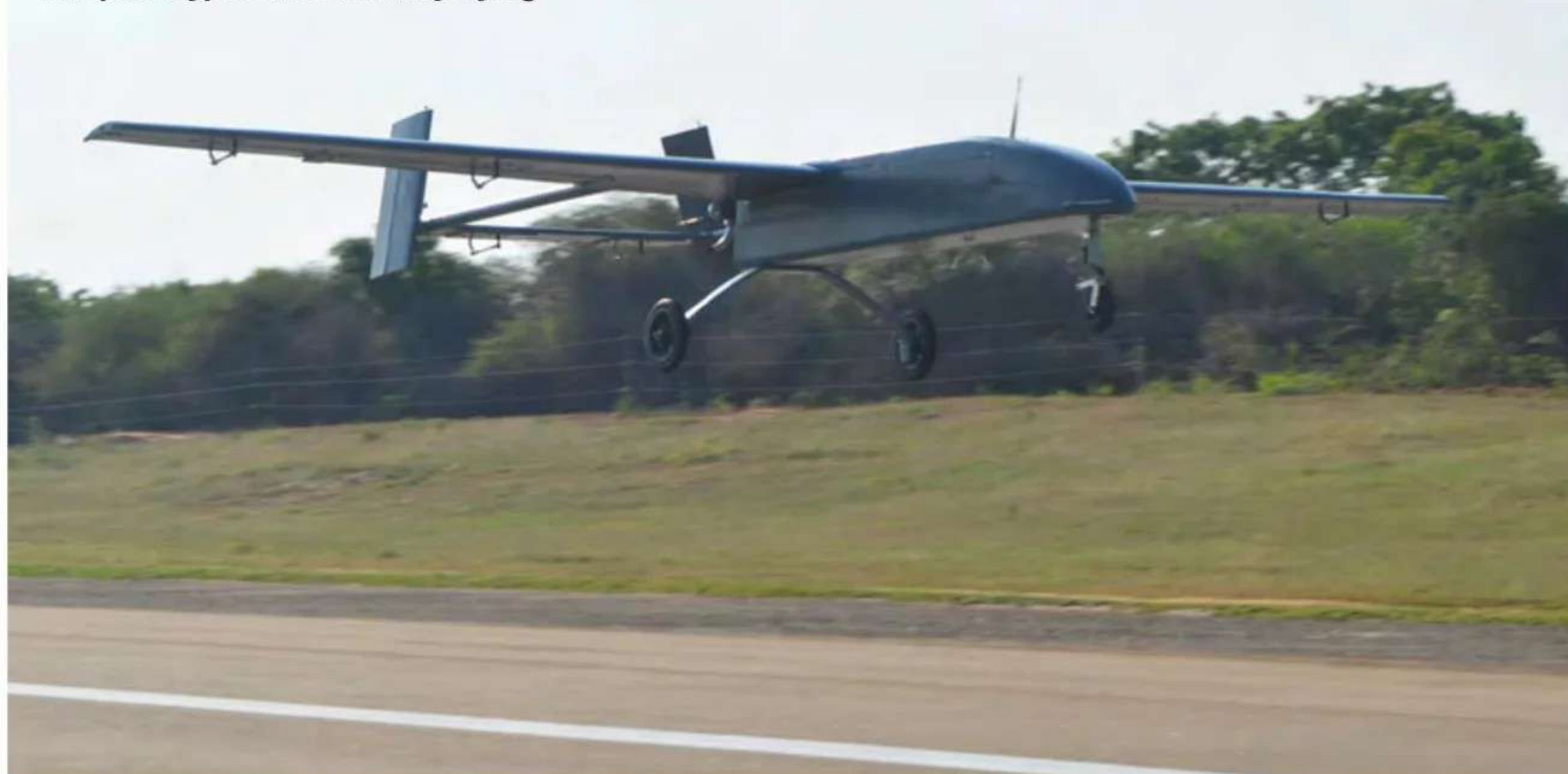
The SLAF developed the Lihiniya unmanned aerial vehicle (UAV) with a planned range of up to 150km. Two prototypes are currently flying
